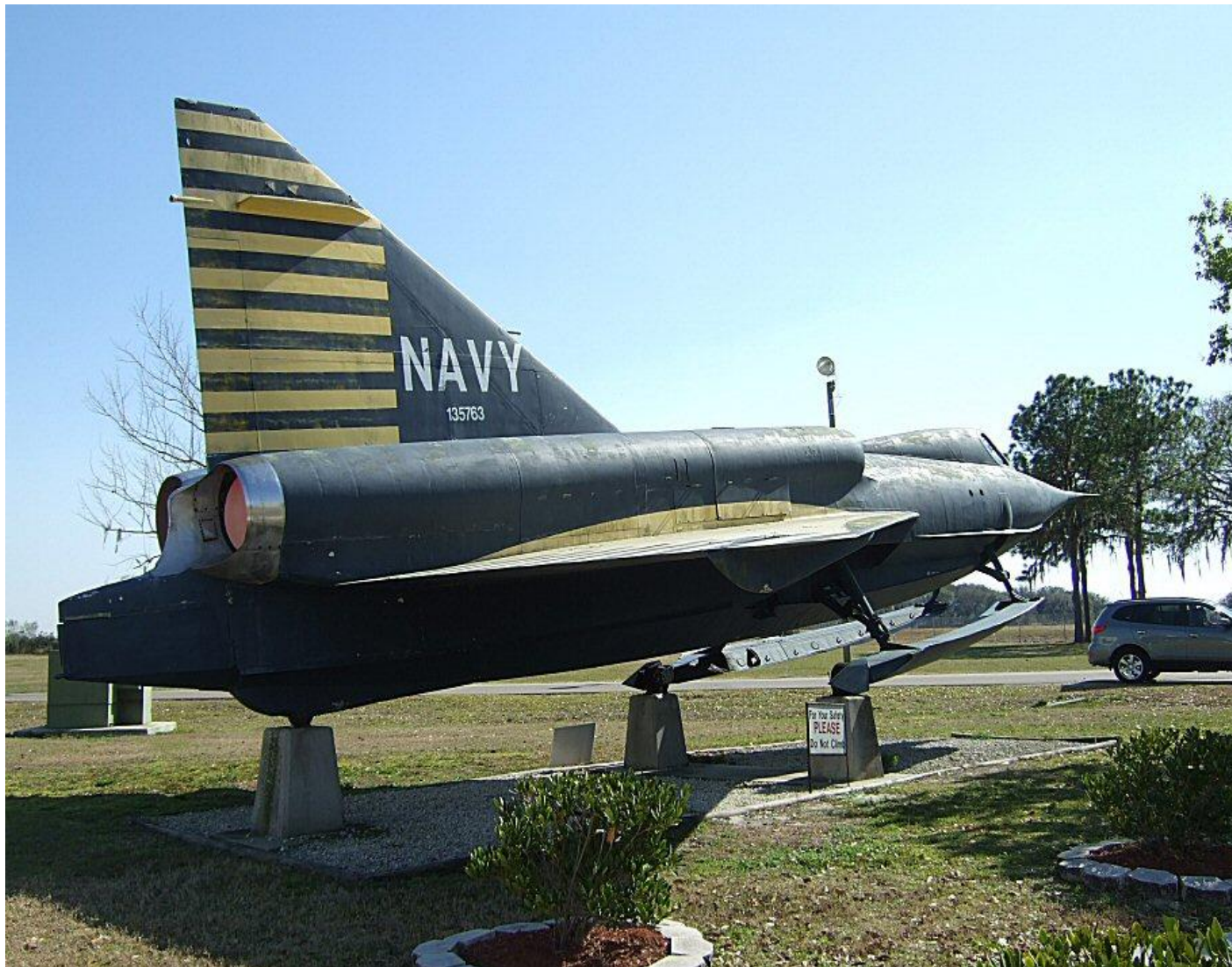
An example of a “Delta” wing, shown here on the US Navy Sea Dart at the Florida Air Museum on the grounds at Sun-n-Fun. Photo: Debey Von
