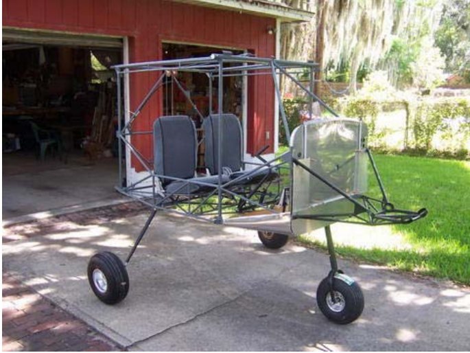
Tim Sweeney's Rans S-6 project—cabin structure and firewall mounted on landing gear.
